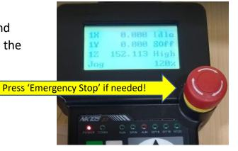
14. Upon completion of the program the router will return 'home' and then 'park' itself at the back left corner of the machine bed. You can interrupt this by pressing the stop button on the handset.
