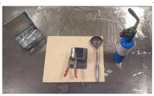
Remove all flammable materials with the exception of the pouring board.
