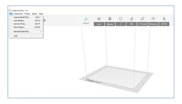
3. By default, the parts should be positioned correctly when imported and manipulation is likely not required. If it is, click on the model and manipulate it using the hoops such that it will not require 'supports' to successfully print. If you did move the model, make sure it is 'laying flat' on the build plate by using the 'Lay Flat' button at the bottom of the window!
