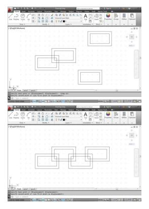
Now use the Trim command to remove the pieces out of the lines to give the appearance that the links are connected to
