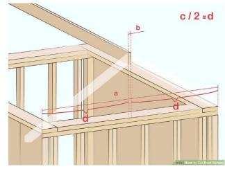
4) Roof pitch. The pitch of the roof is a ratio: the number of inches that the roof rises vertically for every foot of roof. This is a way of measuring the degree of steepness of the roof. If the roof rises 5 inches for every 1 foot, its pitch would be written as 5/12.
