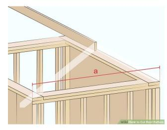
2) Subtract the width of your ridge beam. The ridge beam is the vertical piece of wood which will form the peak of the gable, and to which you'll fasten the rafters on either sides. Measure the width of the ridge beam: it should be 1 ½" (2 x 4 or 2 x 6). Subtract this measurement from the width of your building.
