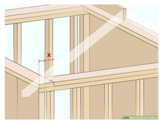
4) Position the body of the framing square on the rafter. Use the body (long side) of the framing square. Rotate it 180° from how you've been using it (so the right angle is pointing up). Set it so that the 8-inch mark on the body of the framing square intersects the line for the tail cut. This will provide a 4 in birdsmouth cut. Use your pencil to trace this line onto the wood.
