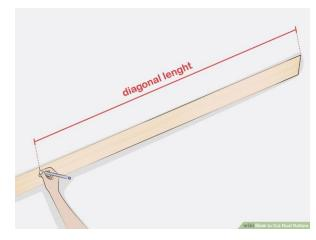
The "line Length" or diagonal measurement is the full length of the rafter, minus the overhang. Measuring the "line length" or diagonal length will allow you to make the tail and bird's mouth cuts in the correct locations.
