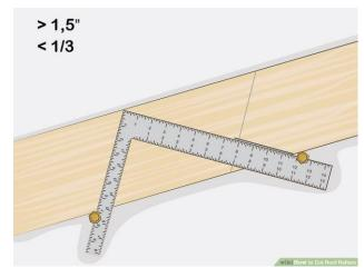
If your bird's mouth cut is not 4 inches deep, slide the framing square to shorten or lengthen the length of the cut accordingly. The rule for a birdsmouth is that it should be 1/3 of the width of the wood you are working with. So, if you are using a 2 x 4 as a rafter, the birdsmouth depth should be just under  $1 \frac{1}{7}$  in depth.
