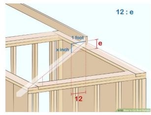
5) Calculate the rise of your roof. The "rise" is the vertical measurement that indicates how tall the roof will be at its highest point above the walls of the building. The rise is the exact height of the ridge beam.
