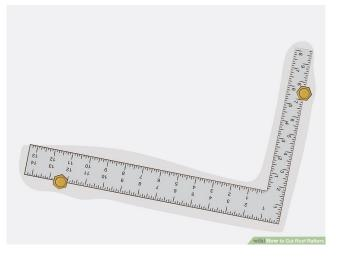
2) Mark the plumb cut Line at the top of the rafter. The plumb (or ridge) cut is made at the top of the rafter. Choose which end of your rafter you want to be the top. Set the framing square on top of the rafter beam, with the tongue facing the top of the rafter. Then, use a pencil to trace the outside edge of the framing square's tongue.
