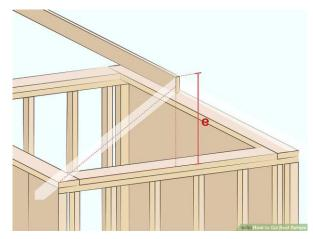
6) Determine the line length of each rafter. To calculate the "line length" you use
