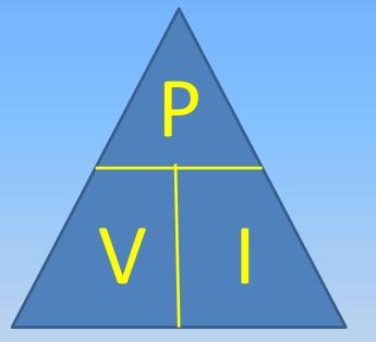
P = Watts, V = Voltage, I = Current
