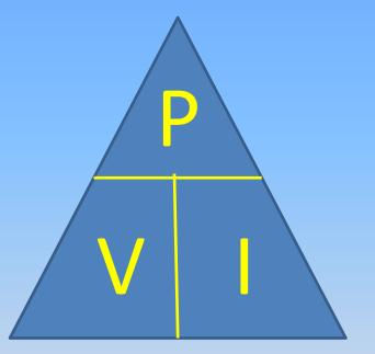
P = Watts, V = Voltage, I = Current  $P = V \times I$  I = P / V V = P / I
