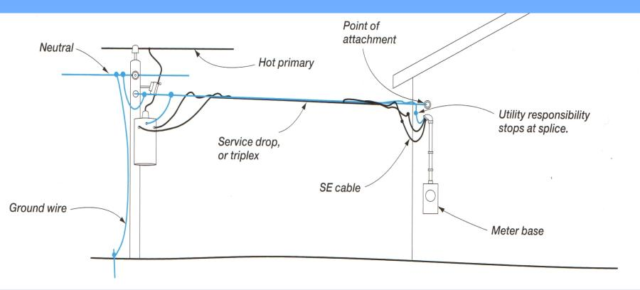
Notice the "Ground wire" attaching to the neutral wire at the power pole and then into the ground. This is to prevent electrocution.
