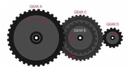
A compound gear train consists of two gear trains (gear A/B and gear C/D) that are joined together. Notice how gears B and C are joined together on the same shaft. By doing this, you can configure different gear ratios.
