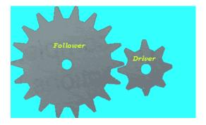
For every 5 time the little gear goes around, the bigger gear goes around 1 times.
