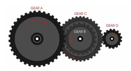
You now have the 2 gear ratios figured out. To find the <u>final</u> gear ratio you simply multiply the ratios together;
