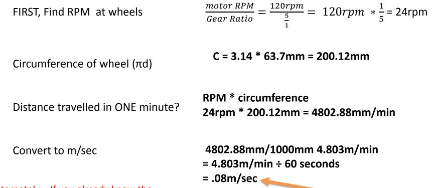
Alternately – If you already know the speed the wheel is going in m/s (previous slide .4m/s), then simply divide the speed by the gear ratio
