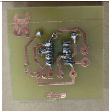
Solder all three components in place. Make sure the solders do not touch each other
