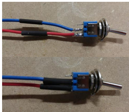
Solder wires to the switch. Notice the heat shrink on the wires first 😊 Make sure you do not burn out the switch by holding the solder pencil TOO LONG on the switch legs.
