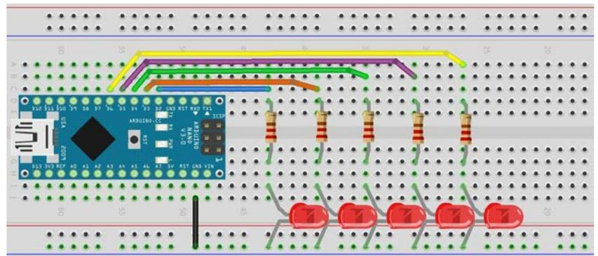
3. The code you used in Lab 1 needs to be expanded to have all 5 LEDs work. Start adding to the code by initializing D2-D6 in the Setup using `- pinMode(xx, OUTPUT);` Next, in the main part of the program, add 4 more `digitalWrite(xx, HIGH);` and 4 more `digitalWrite(xx, LOW);` lines to your code so that ALL 5 LEDs blink on and then off. Finally, change the delay to be only 250ms. The picture to the right shows the completed code.
